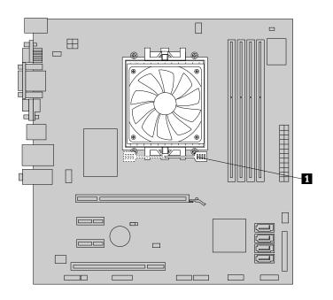
Figure 31. Removing the heat sink and fan assembly
